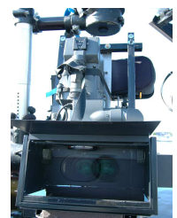
A pair of DigiPrimes on the mirror rig
